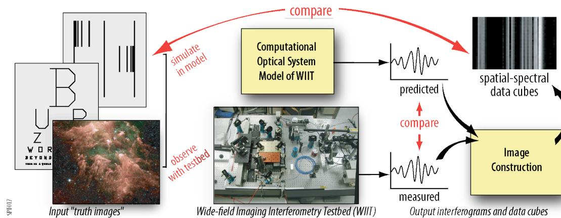
Figure 1. We apply an error-tracking experimental approach in which increasingly complex, more astronomically realistic test scenes are observed, and different observing modes are explored to learn the practical limitations of wide-field spatio-spectral interferometry and to quantitatively understand how each instrument design parameter impacts the quality of the synthesized hyperspectral image cube.
