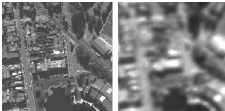
Figure 4 - Left: Object scene used in simulations; Right: Image blurred by system OTF with 0.25 wave RMS unknown pupil aberration
