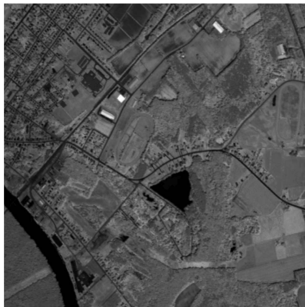
Fig. 2. Panchromatic representation of multi-spectral object. The object consists of 11 spectral bands, centered about 1 \mu\text{m} and spanning 96 nm.
